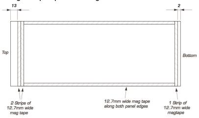
Apply mag tape to straight panels according to the diagram (all dimensions are approx).
