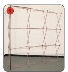
Add the mag bars onto the frame, vertically for front and D-end panels. Then add horizontal mag bars across the top and bottom of the frame.
