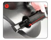
Place the graphic hole though the locator on the base
